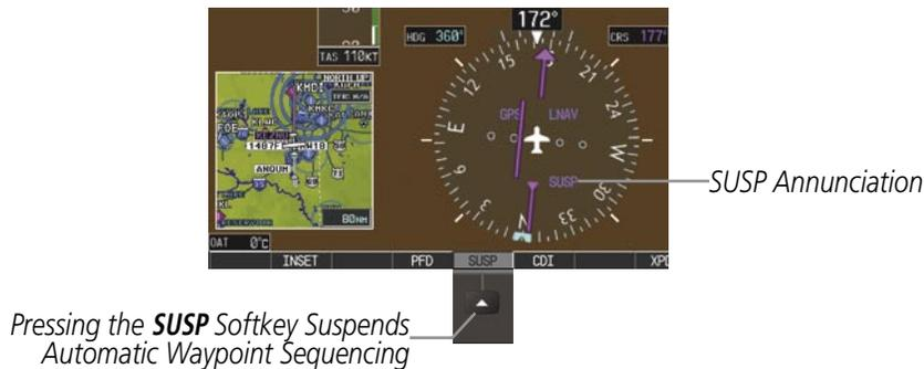
Figure 2-29 Suspending Automatic Waypoint Sequencing
