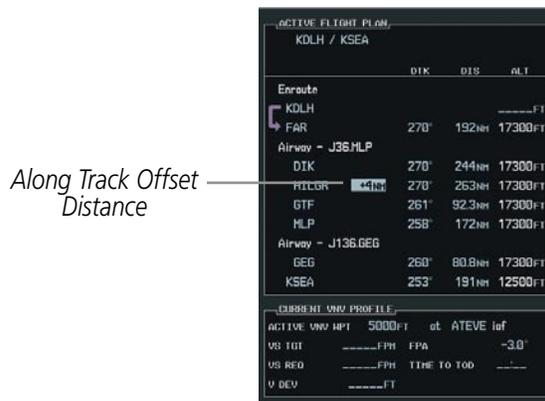
Figure 5-84 Along Track Offset Distance
