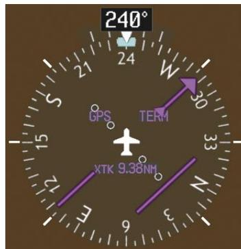
Figure 5-86 Assigned Heading of 240°
