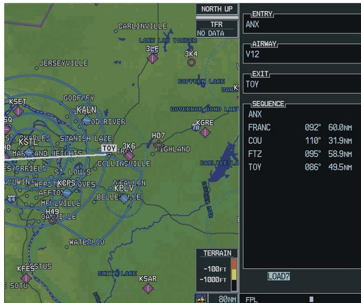
Figure 5-75 Loading the Airway into the Flight Plan
