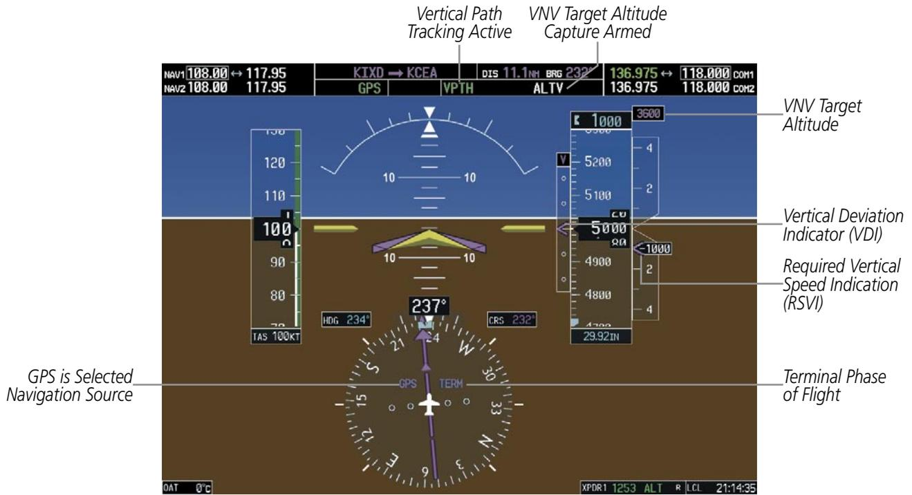
**Figure 7-12 Vertical Path Tracking Mode**
