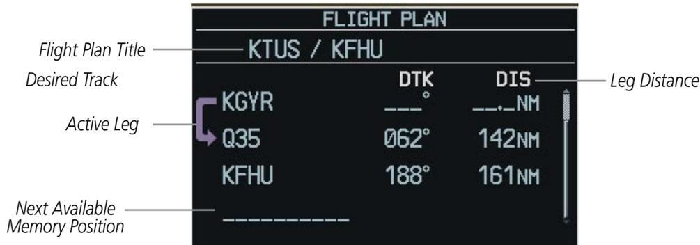
Figure 5-131 Flight Plan Window
