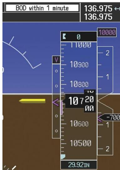
Figure 5-114 Approaching Bottom of Descent (BOD) at OPSHN
