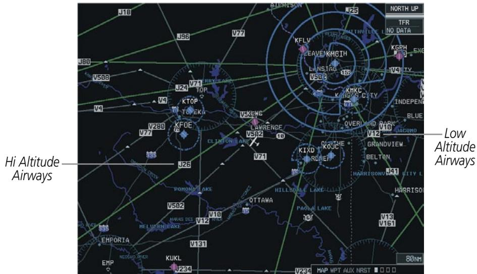
**Figure 5-11 High and Low Altitude Airways**
