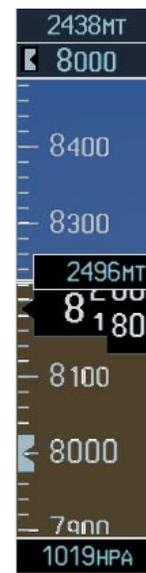
**Figure 2-10 Altimeter (Metric Units)**
