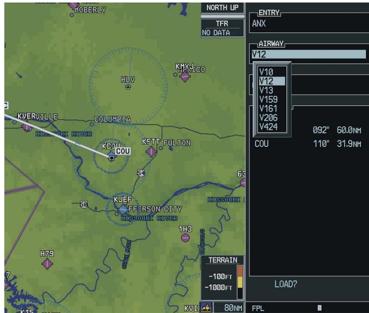
Figure 5-72 Selecting an Airway
