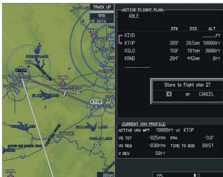
Figure 5-68 Storing a Flight Plan
