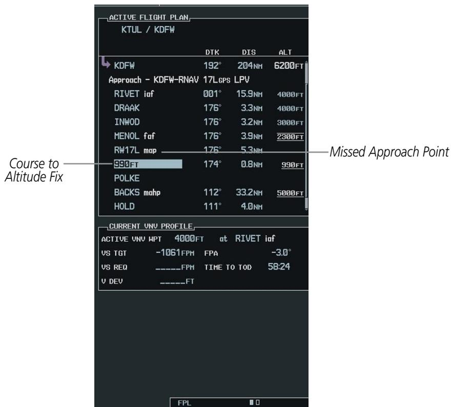
Figure 5-143 Course to Altitude Fix Special Condition
