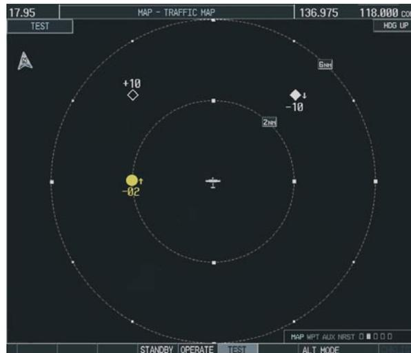
Figure 6-60 Self Test OK Display
