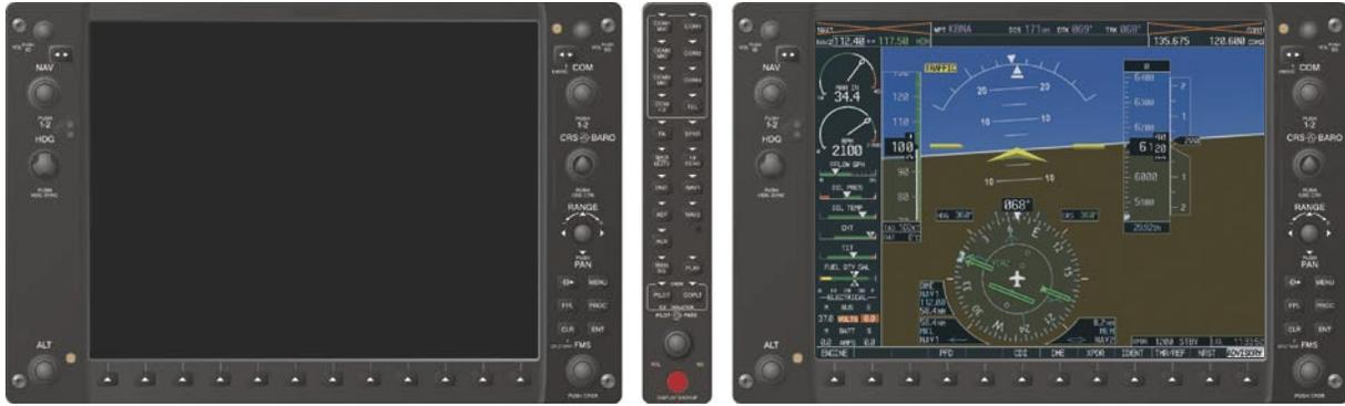
Figure 1-9 Reversionary Mode (Failed PFD)
