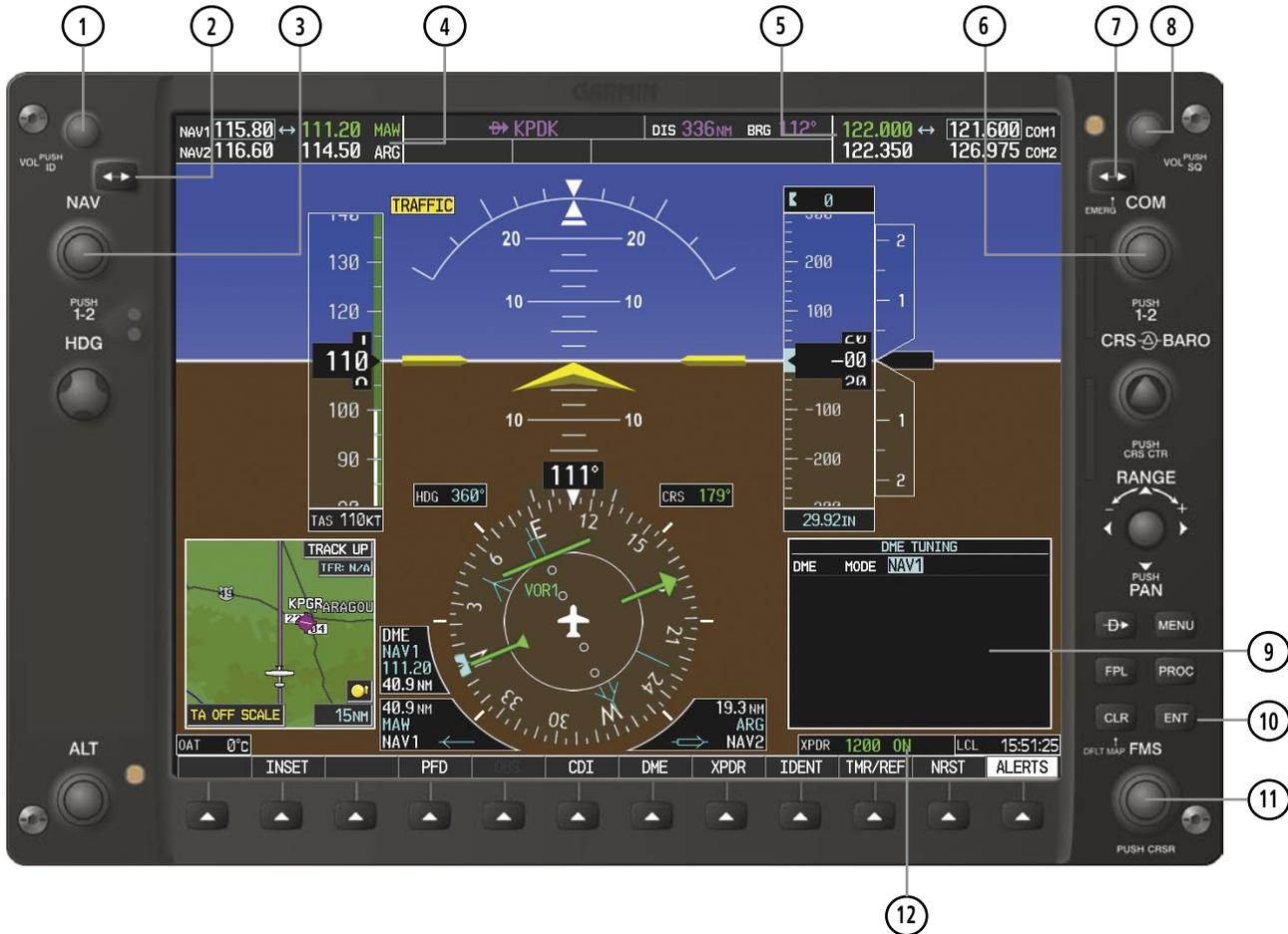
Figure 4-1 PFD/MFD Controls, COM/NAV Frequency Tuning Boxes, and DME Tuning Window (Cessna 172 PFD Shown)
