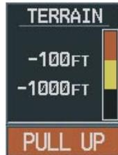
**Figure 6-51 Alert Annunciation on the MFD**
