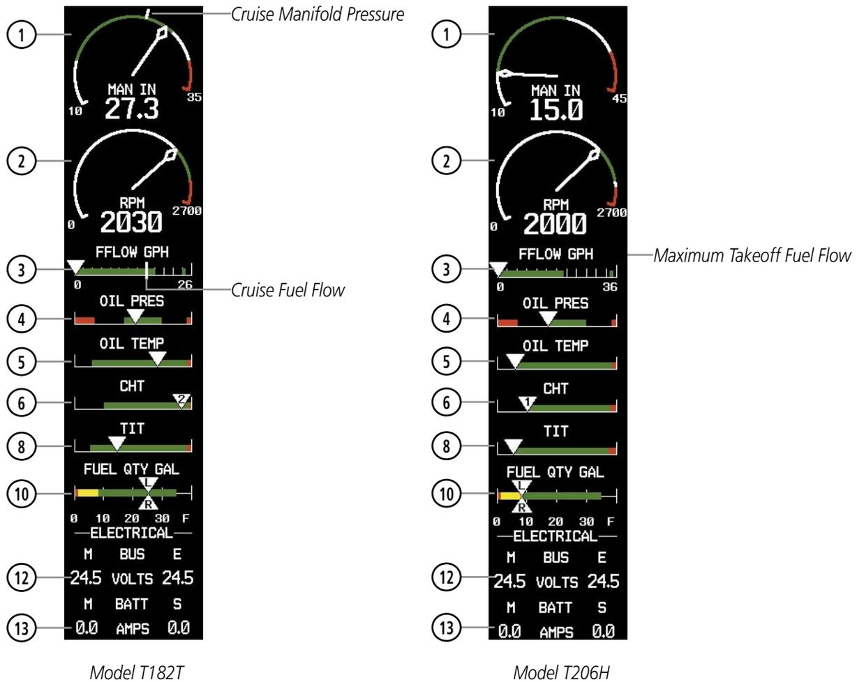
Figure 3-3 Engine Display (Turbocharged Aircraft)
