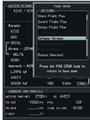
Figure 5-79 Collapse Airway Feature
