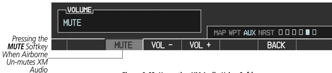
Figure 8-62 Un-muting XM Audio Using Softkeys
