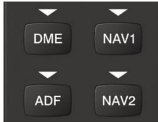
Figure 4-18 Selecting a NAV Radio Receiver
