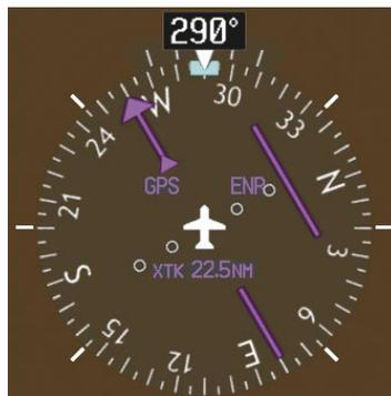
Figure 5-87 Assigned Heading of  $290^{\circ}$
