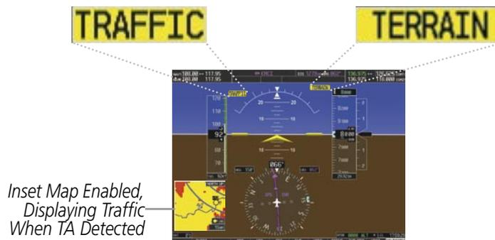
Figure 2-38 Traffic and Example TAWS Annunciations
