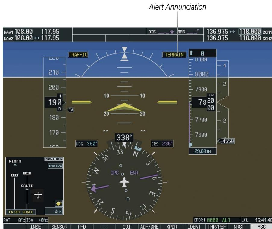
**Figure 6-52 Alert Annunciation on the PFD**
