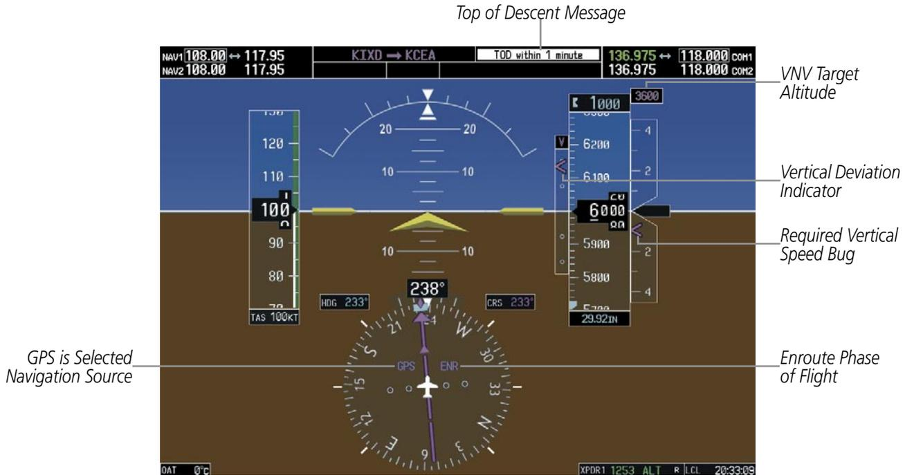
Figure 2-35 Vertical Navigation Indications (PFD)
