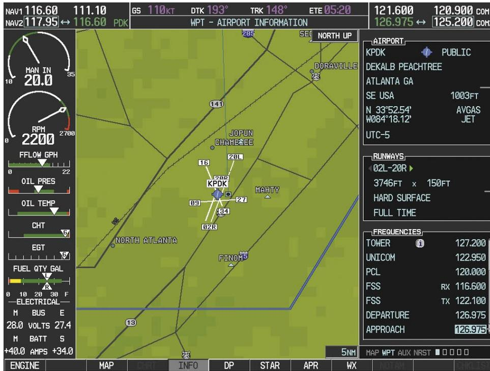
Press **Frequency Transfer** Key to Load Frequency into COM Active Frequency Field
