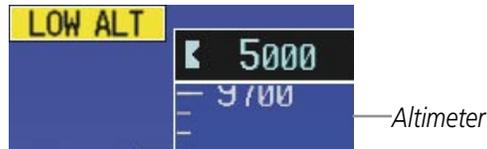
**Figure 2-39** Low Altitude on GPS WAAS Approach
